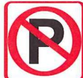
R30 24X24" Barricade mounted, placed on both sides of the street 20' apart ~~2HR~~ prior to start of work.
